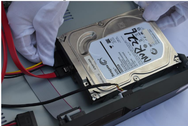
Figure 2-3 Install hard disk
