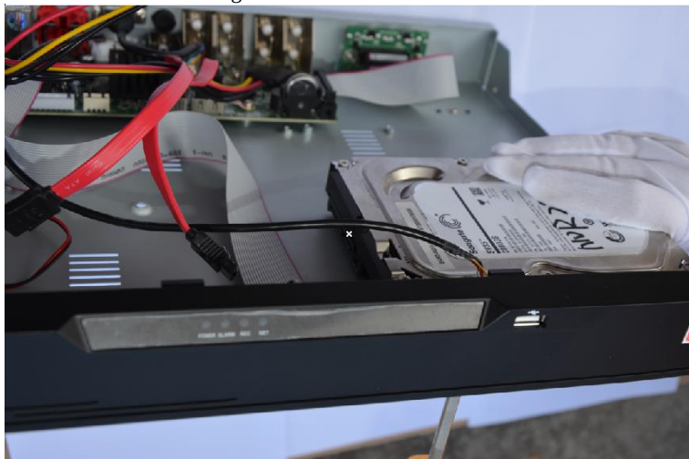
Figure 2-2 Install hard disk
